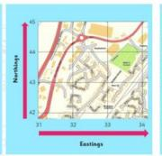
Using the 2 digits of the easting and the 2 digits of the northing creates a four-figure grid reference. This is the reference for the bottom left corner of a square on the map. This makes it easier to search the map for features.
